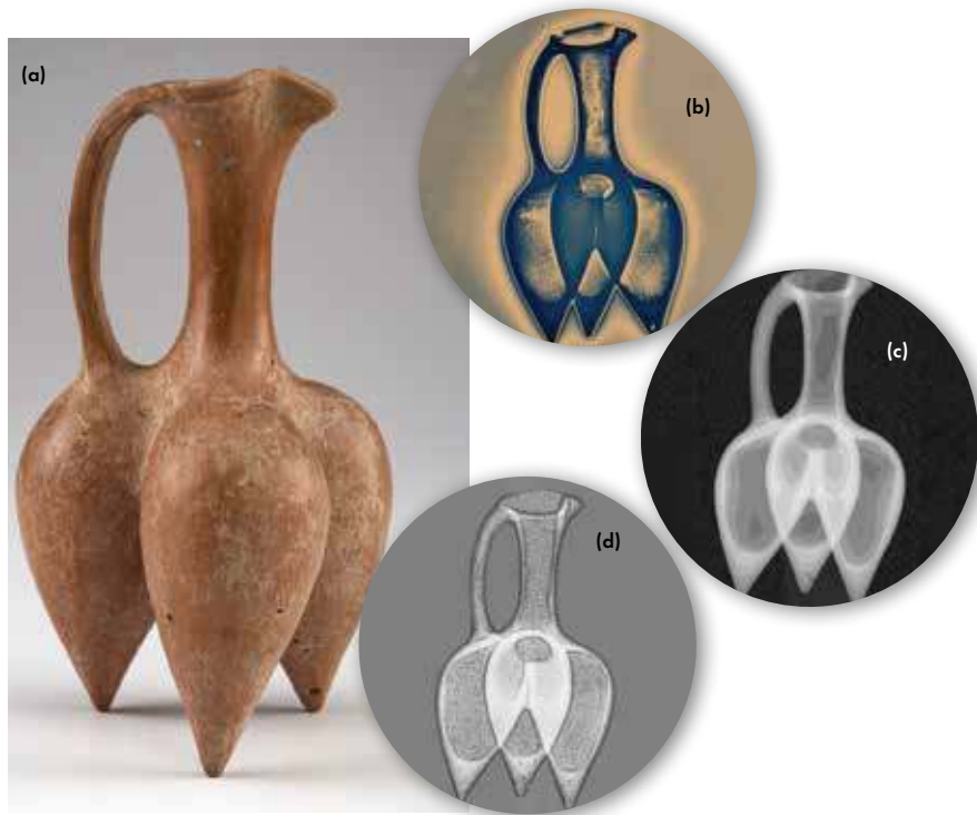
Figure 3. a) Tripod ewer, ca. 1350–800 BCE, Northwest Iran H x W x D: 21.6 x 11.5 x 12.2 cm (8 1/2 x 4 1/2 x 4 13/16 in) Arthur M. Sackler Gallery S1998.169. b) Xeroradiograph (55KV, 5mA, 60 seconds), image reversed for easy comparison. c) Computed radiograph. d) Computed radiograph after digital processing with Adobe Photoshop (Adjust levels to expand channels used, filter: Find edges, adjust levels to expand channels used a second time).
