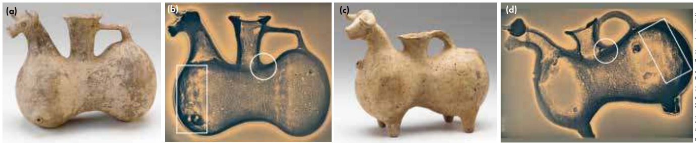
Figure 2. Zoomorphic rhytons (drinking vessel), Northwest Iran, Parthian period ca. 160 BCE–224 CE, and side-view xeroradiographs (acquisition conditions: 75 KV, 5 mA, 1 minute). Arthur M. Sackler Gallery. a,b) S1987.94 (H x W x D: 20.3 x 25.6 x 14.1 cm); and c,d) S1987.95 (H x W x D: 23 x 29.2 x 12.3 cm). Square around mottled area; circle around neck join.
