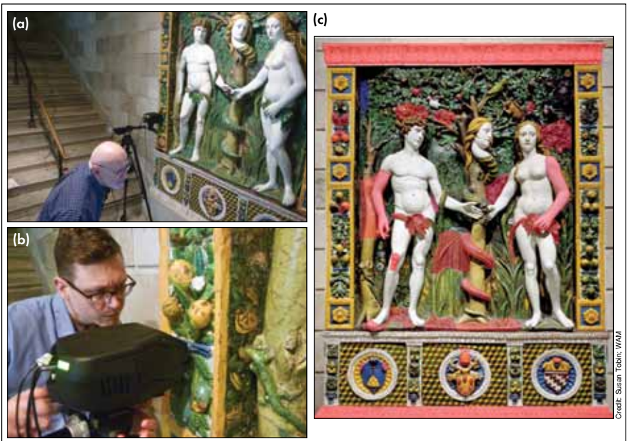
Figure 5. (a) and (b) A portable XRF spectrometer analyzed the glazed surface of the life-sized Adam and Eve (WAM No. 27.219) (280 cm high) created by Giovanni della Robbia in Italy circa 1515. (c) The red shadowing indicates areas of suspected restorations, which were confirmed by XRF.
