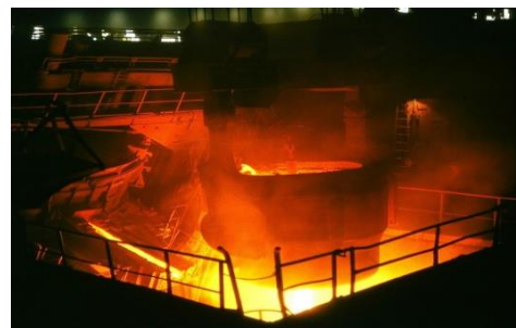
Figure 2. Steelmaking – refractory materials are used in the crucible.
