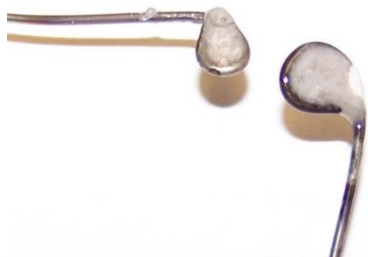
Figure 6. Beads that have a gray, milky color rather than a transparent, bright color due to the gas bubbles that remain trapped in the amorphous borax.
