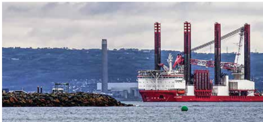
MPI Adventure, a wind turbine installation vessel, anchored off Luke's Point, Bangor, Belfast Lough, Northern Ireland.
