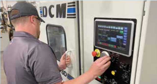
Modern rotary surface grinders like those from DCM Tech offer advanced sensors and controls that can reliably achieve tighter dimensional tolerances, flatness, parallelism, and surface finish in much less time. Credit: DCM Tech
