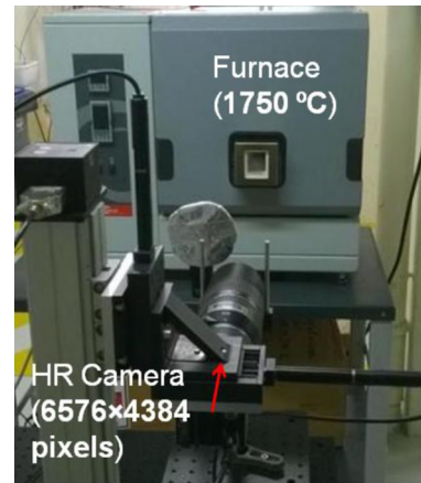
Fig. 8. High-temperature furnace with a high-resolution camera.
