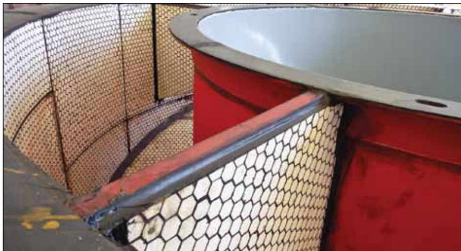
Trelleborg Engineered Systems (Brisbane, Queensland) manufactures a variety of products, including those related to mining and mineral processing. One example is this cyclone underflow launder for iron ore, which is lined with glue in ceramic mats.
