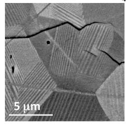
centrosymmetric structure with ferroelastic domains and polar properties.
