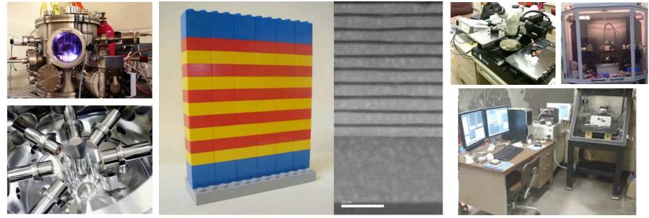
We use off-axis RF Magnetron sputtering to make very finely layered ferroelectric superlattices, which we characterize by XRD, TEM, AFM, electrical measurements, etc. We are also heavy users of the NSLS and the CFN at BNL.
