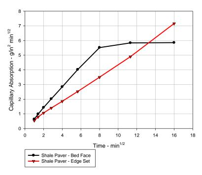
For extruded brick, it is not uncommon to see a higher absorption rate parallel to extrusion with a lower saturation level due to the alignment and connectivity of pores.
