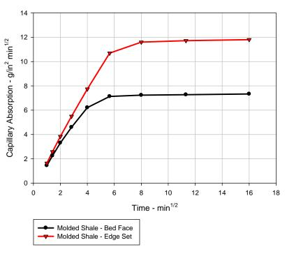
For molded brick, we do not see as much difference between the orientation directions.
