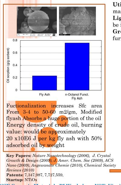
**Utilizing:** Surface Engineering approach to Flyash – for making Oil Absorbent
