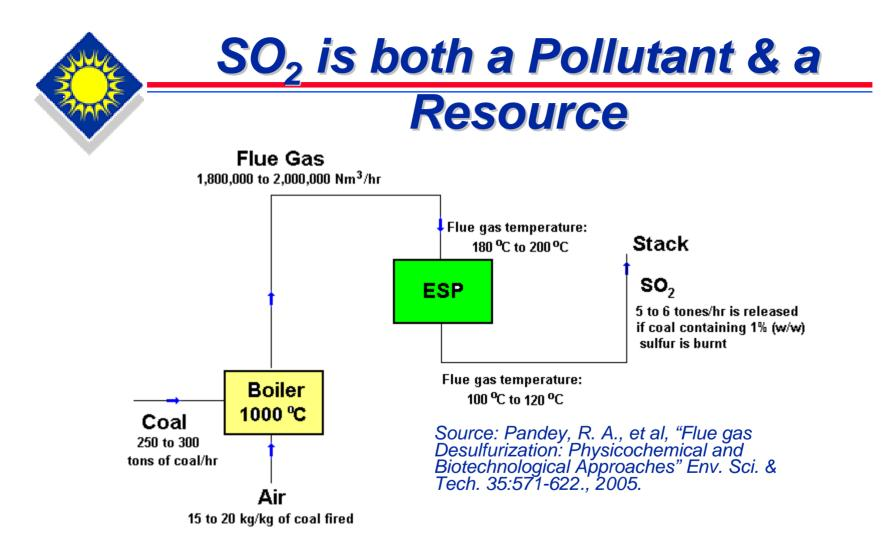
Generation of  $SO_2$  in 500 MW coal fired power plants can produce huge amounts of  $SO_2$  that can be used for the production of  $H_2$  as well as fertilizers.
