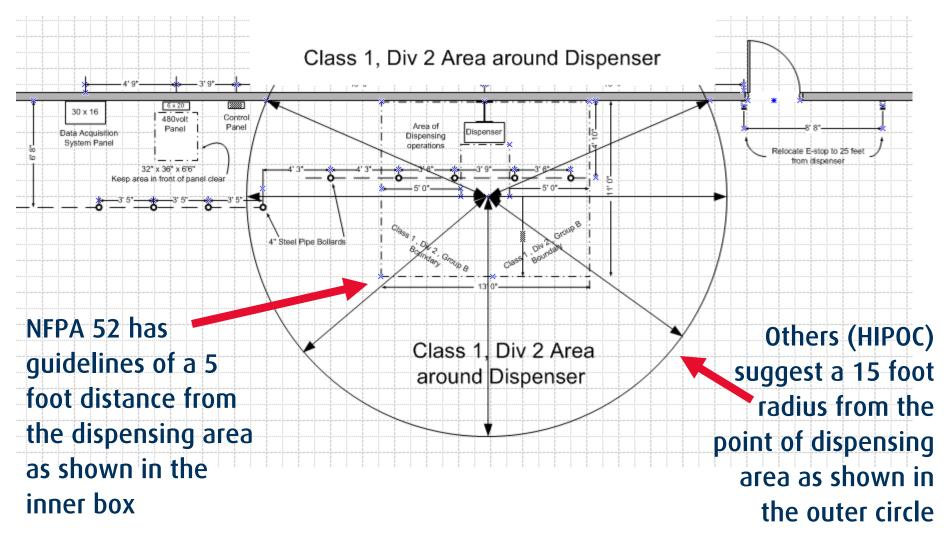
Interior walls, doors, and window openings within 15 feet (4.6 meters) of the dispenser shall be constructed of non combustible materials. No storage of combustibles
