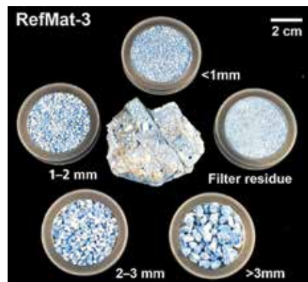
Sample material RefMat-3 before (center) and after fragmentation and subsequent classification by grain size.
