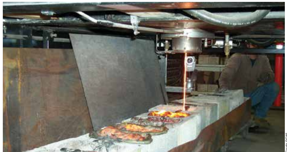
Fig. 2. Melt drops out the bottom-pour electric furnace into collection pots.
