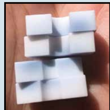
Figure 3. Ring sample cross sections demonstrating nucleation-based discoloration extending far below the original surface. Credit: Elcon Precision
