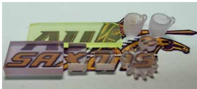
Highly transparent yttrium aluminum garnet (YAG) ceramics with 3D structures, created via a lithography printing method.
