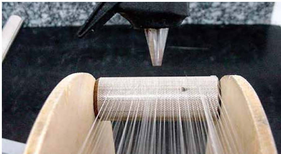
Rafael Salomão and Victor Pandolfelli used a hot-melt glue-gun and rotating barrel to create thin continuous fibers from dense polymeric rods, which they then added to refractory castables to prevent spalling.
