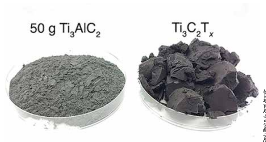
Images from Gogotsi's group of the precursor Ti_3AlC_2 MAX (left) used in synthesis of 50 g Ti_3C_2T_x batch (right).
