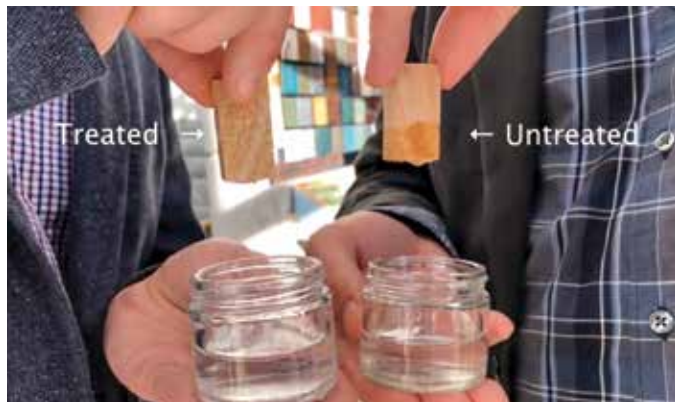
By treating wood using atomic layer deposition, Georgia Tech researchers found they could manage moisture content, mold growth, and thermal conductivity.
