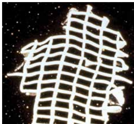
Figure 2. Results from the first extrusion of cellular ceramic (left), and drawings from the patented idea filed in November 1971. First tested in July and first scaled in October 1971.
